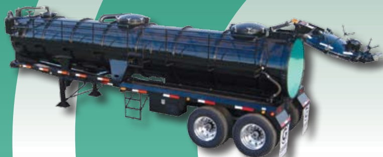
107 BBL – Vacuum/Dump for Closed Loop Systems
