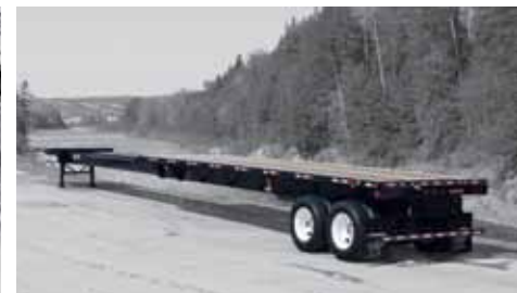
Galvanized rear sill with closed bumper
