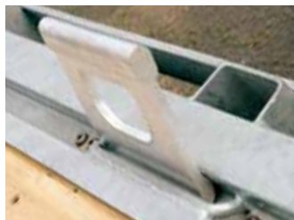
Unique cargo securement anchor point (cargo hand style) Galvanized side rails
