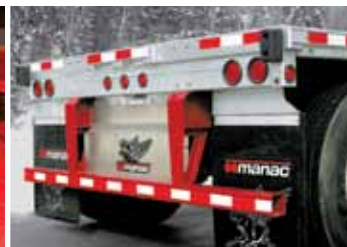
Galvanized rear sill with closed bumper
